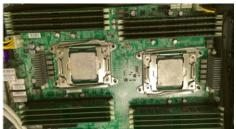
Need to install 02 CPUs and all Memory slots. If no display it might be 1 of memories slot defective. Also Connecting the Eth Cable to Management Port. Will get display right away.
