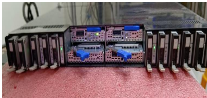
57-3 SSD stress test 時確認 SSD LED 有閃爍
